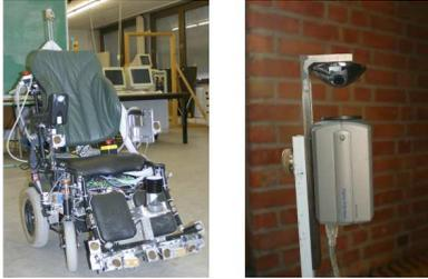
**Figure 1:** Left: the robotic wheel chair platform. Right: the omnidirectional camera, composed by a color camera and an hyperbolic mirror.
