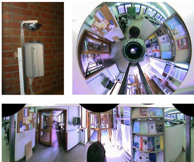
**Figure 2: omnidirectional camera system (top left), example omnidirectional image (top right), transformed image (bottom.)**
